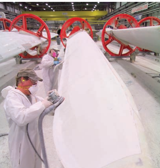
Workers smooth the surface of blades manufactured at Gamesa USA's Ebensburg facility.
