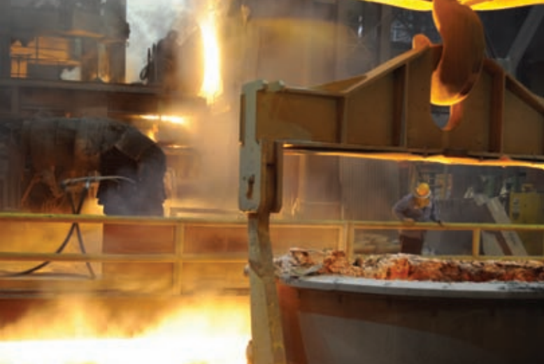
A ladle transports hot metal tapped out of the Electric Arc Furnace.
